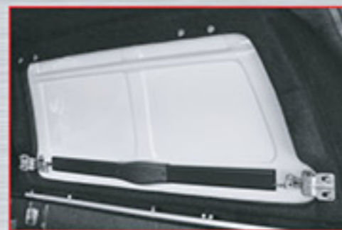
Double Layers Fiberglass Side Doors.
