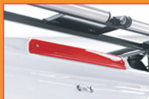
High Mounting L.E.D. Brake Light.
