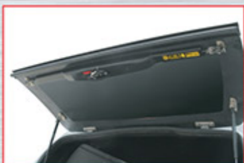
Tinted Rear Door Glass with smooth pressure gas struts.
