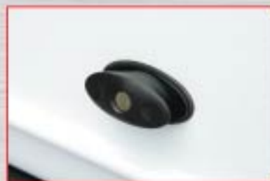
Injected Door Handle with Lock and Key.
